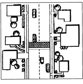
Speed *tables* are flat-topped speed humps that are often constructed with asphalt and may have a brick pattern or other textured material applied on the flat top.
