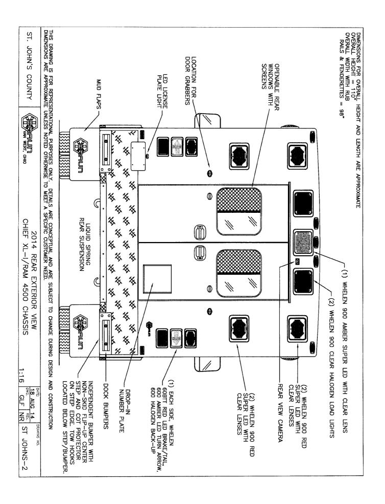
OVERALL LENGTH = 306.5" MODULE LENGTH = 169" DIMENSIONS FOR OVERALL HEIGHT AND LENGTH ARE APPROXIMATE OVERALL HEIGHT = 110" THIS DRAWING IS FOR REPRESENTATIONAL PURPOSES ONLY. DETAILS ARE CONCEPTUAL AND ARE SUBJECT TO CHANGE DURING DESIGN AND CONSTRUCTION DIMENSIONS ARE APPROXIMATE UNLESS NOTED OTHERWISE TO MEET A SPECIFIC CUSTOMER NEED. COMPARTMENT ST. 0.S.S #1 CLEAR OPENING: 81.75h × 17.75w
