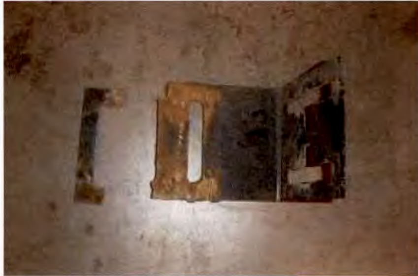
FAILED BUMPER MOUNTING BRACKET (6,940 TEST MILES)
