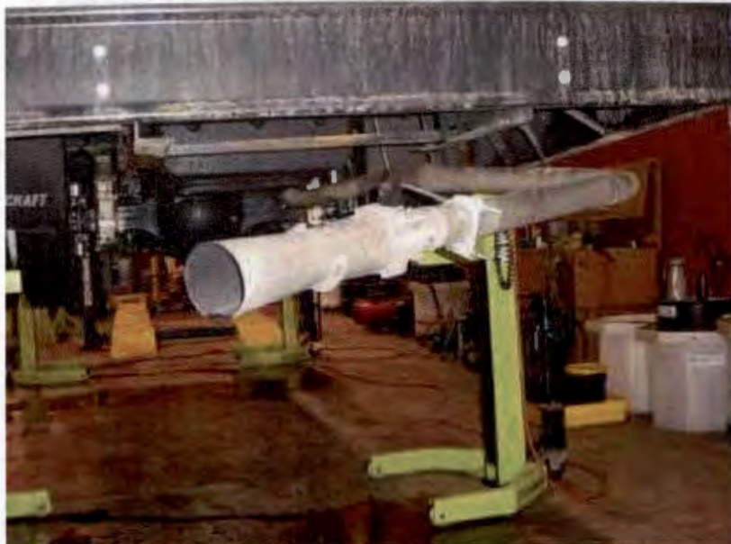
BROKEN TAILPIPE HANGER (6,715 TEST MILES)
