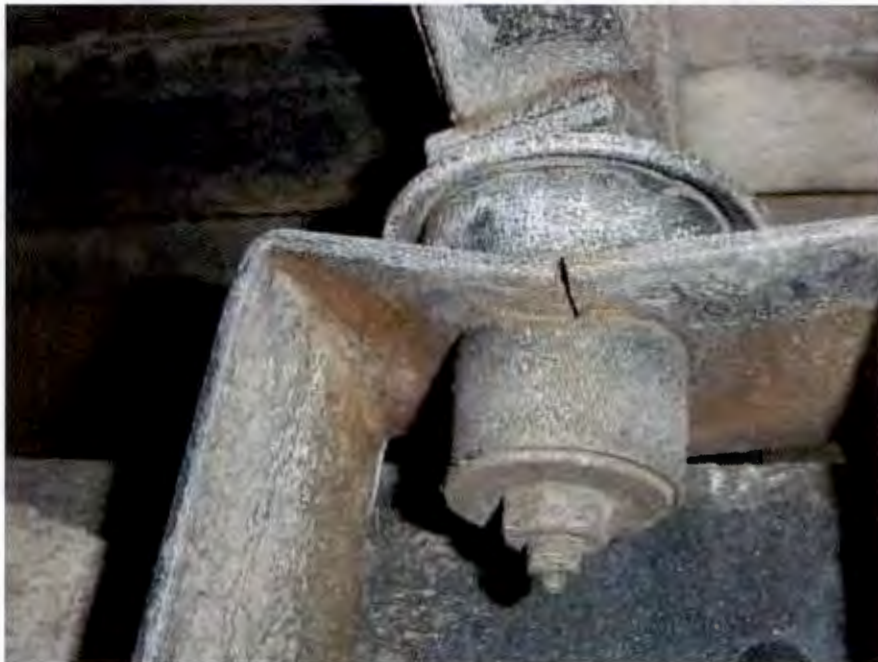
BROKEN BODY TO FRAME BRACKETS (4,045 TEST MILES)
