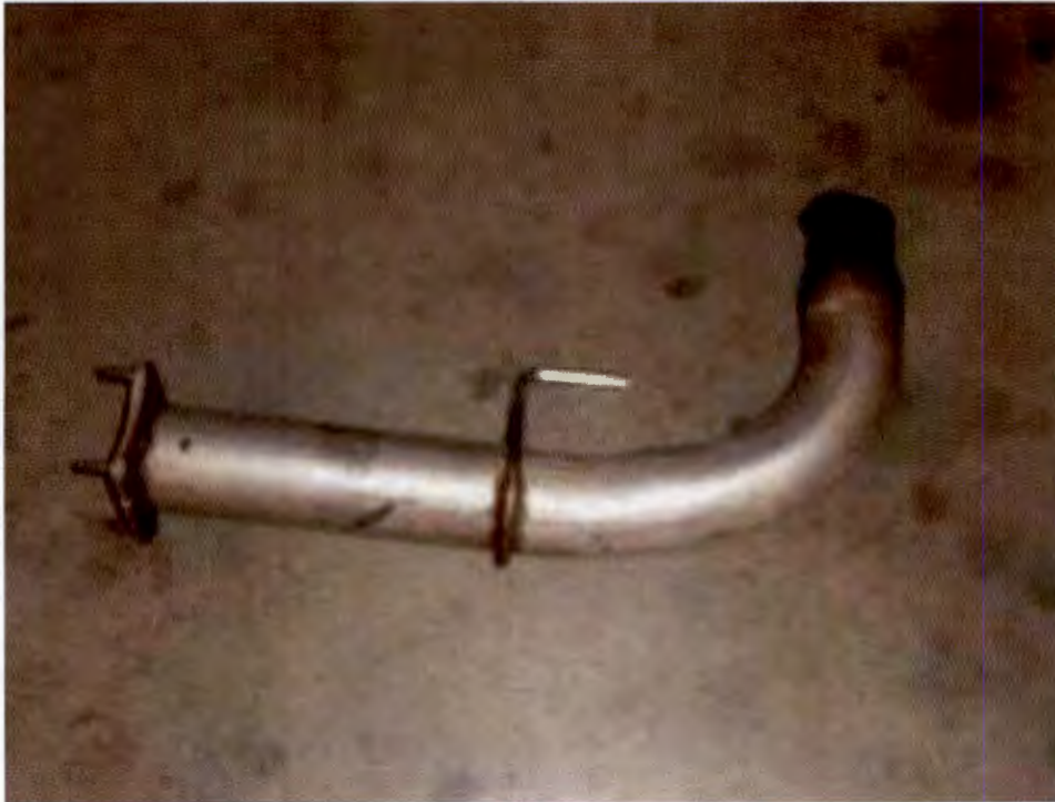
FLANGE CRACKED ON EXHAUST DOWN PIPE (1,642 TEST MILES)
