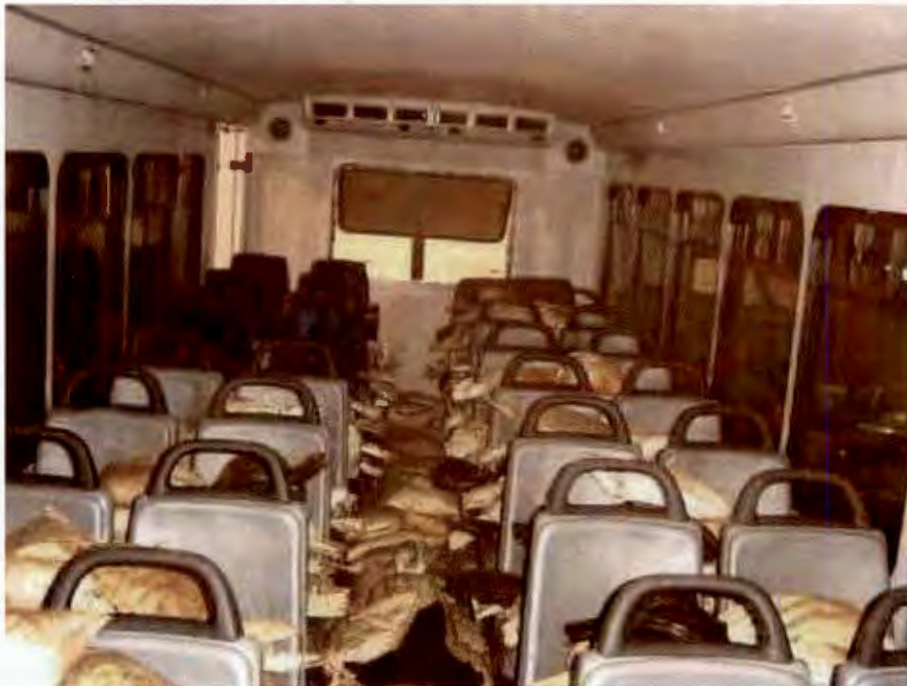
BUS LOADED TO 2.5 TIMES GVL (18,750 LBS)
