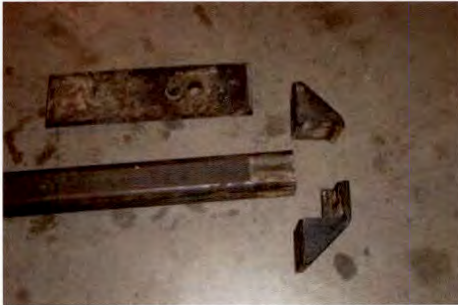
BROKEN LEFT FRONT STABILIZER BAR BRACKET (4,045 TEST MILES)
