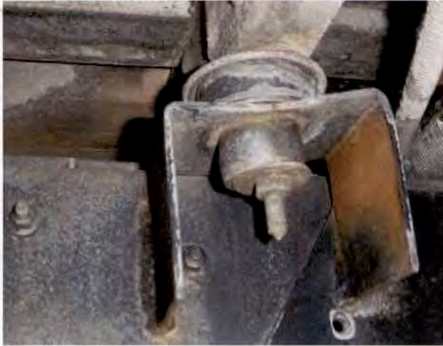
BROKEN BODY TO FRAME BRACKETS (4,045 TEST MILES)
