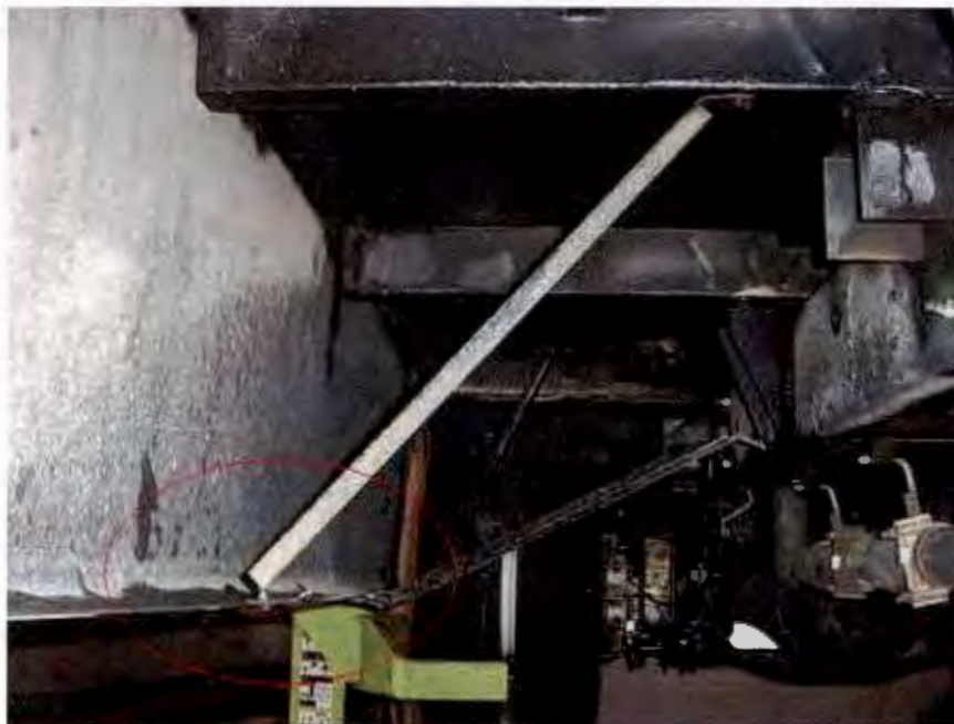
BROKEN BODY PANEL SUPPORT (9,347 TEST MILES)
