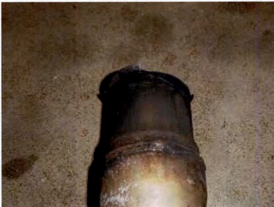
FLANGE CRACKED ON EXHAUST DOWN PIPE (1,642 TEST MILES)
