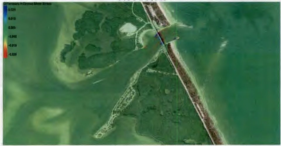
Under contract to Transystems, INTERA assessed the effects of the foundations of the planned replacement bridge over Sebastian Inlet to ensure any change in sediment transport does not interfere with inlet management bypassing practices and features, such as the sand trap inside the inlet.
