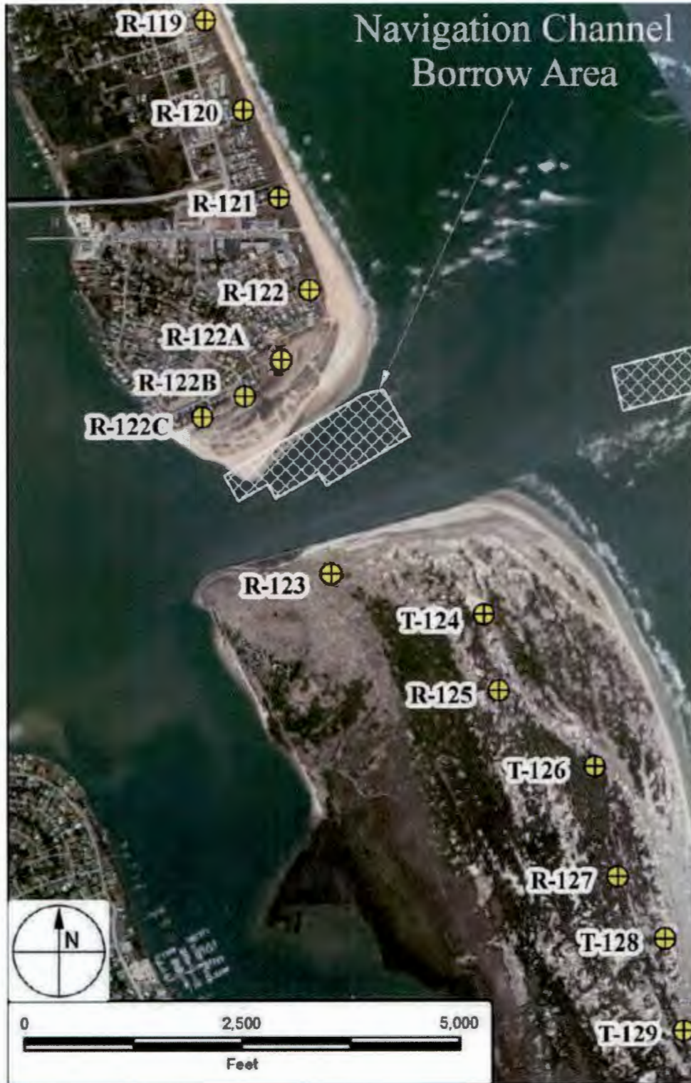
Figure 4: R-Monuments and the 2012 SPP Borrow Area near the Porpoise Point Shoreline (Taylor, 2013)
