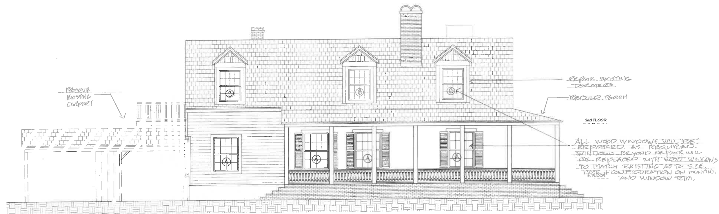
East Elevation 1/4"=1'-0" Existing
