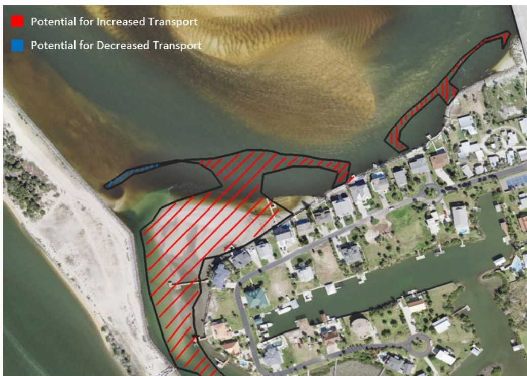
Figure 4.37 Scenario 2 (SHR Deepened to -6 ft NAVD88) Effects on Erosion during Flood Flow
