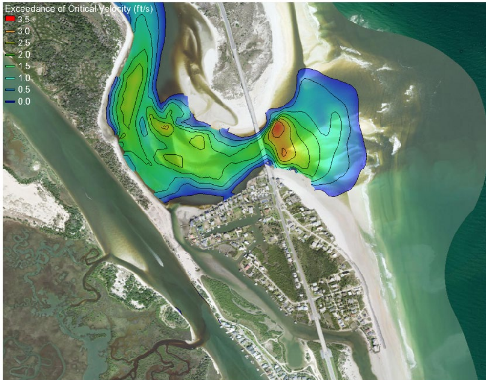
Figure 4.29 Exceedance of Critical Velocity at Peak Flood Flow – Existing Conditions
