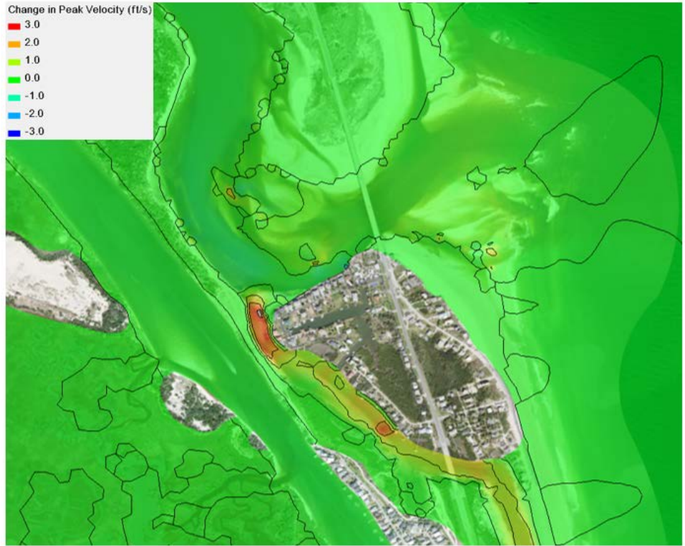
Figure 1.16 Change in Velocity within Inlet at Peak Ebb Flow – Scenario 2 vs. Existing Conditions
