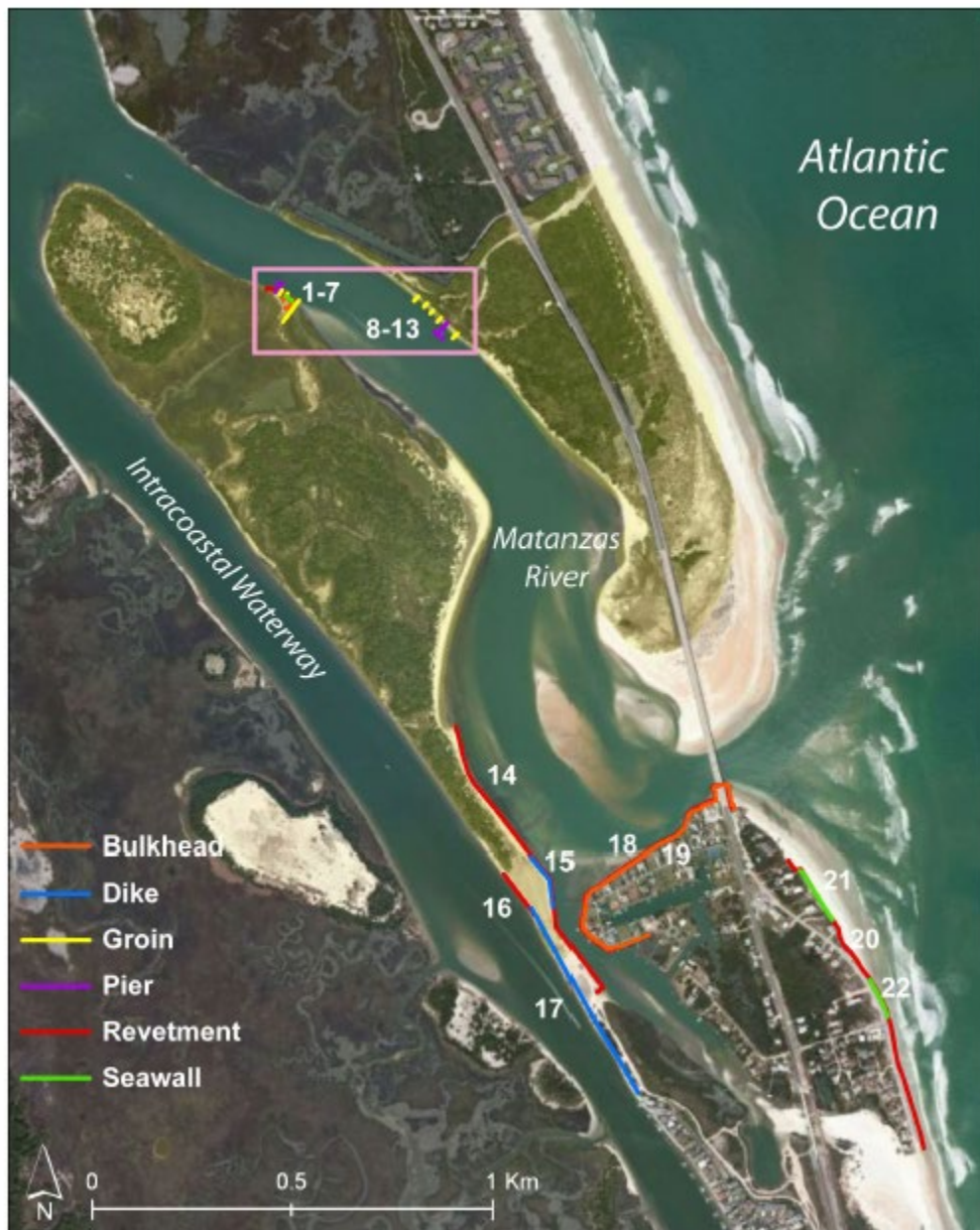
Figure 2.2 Inventory of Coastal Structures in Fort Matanzas Area (NPS, 2013)
