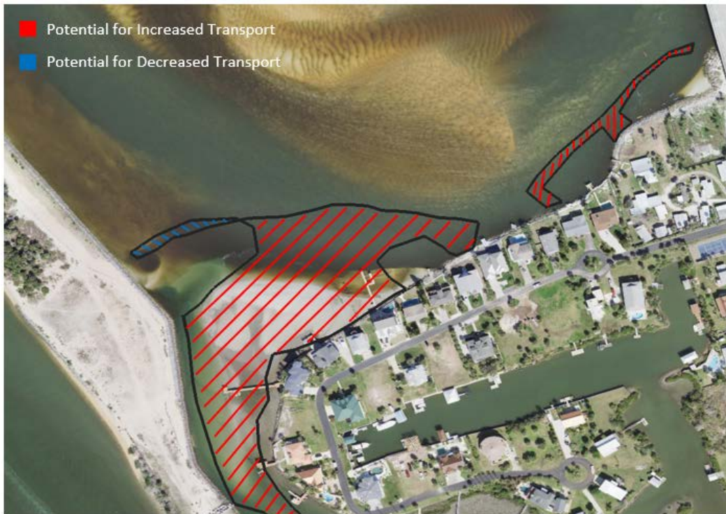
Figure 1.37 Scenario 3 (SHR Deepened to -10 ft NAVD 88) Effects on Erosion during Flood Flow
