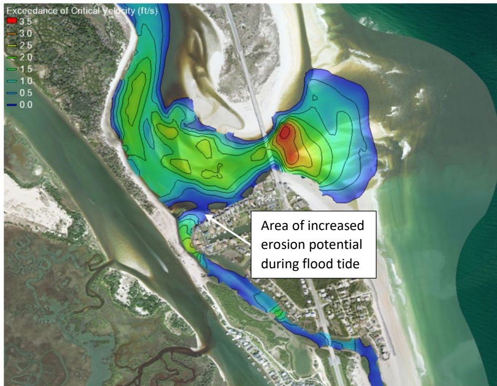
Figure 4.31 Exceedance of Critical Velocity at Peak Flood Flow – Scenario 2 (SHR Deepened to -6 ft NAVD88)
