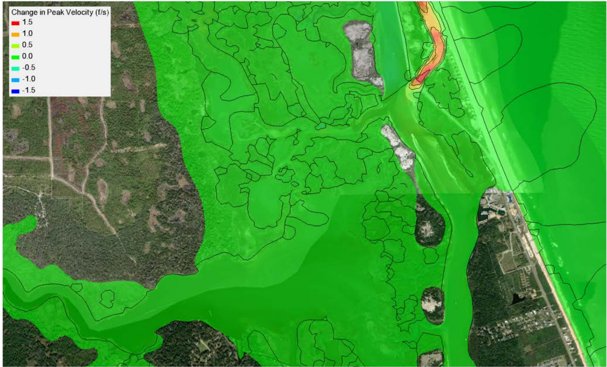
Figure 1.42 Change in Velocity within Inlet at Peak Ebb Flow – Scenario 2 vs. Existing Conditions
