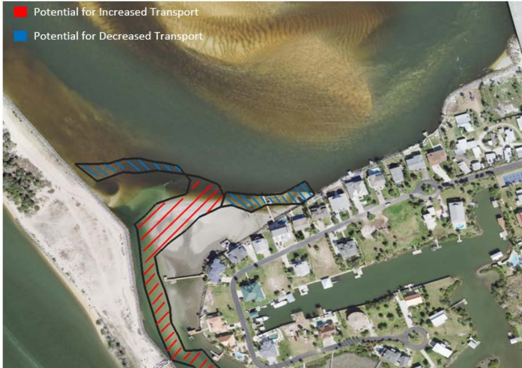
Figure 1.36 Scenario 3 (SHR Deepened to -10 ft NAVD 88) Effects on Erosion during Ebb Flow
