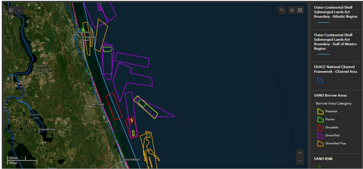
Figure 3.19 Classification of Sand Sources Offshore Southern St. Johns County – Northern Volusia County https://sacs.maps.arcgis.com/apps/dashboards/46d59434896a464a89d1f3b54d43d0d5
