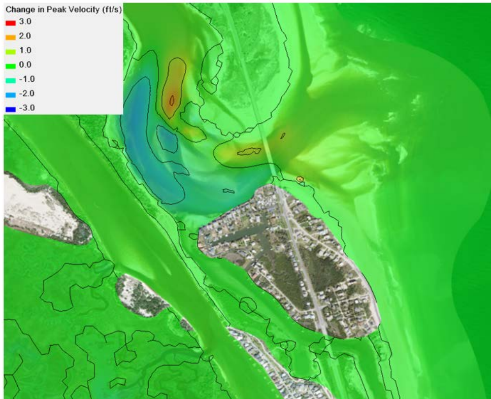
Figure 1.25 Change in Velocity within Inlet at Peak Flood Flow – Scenario 4 vs. Existing Conditions
