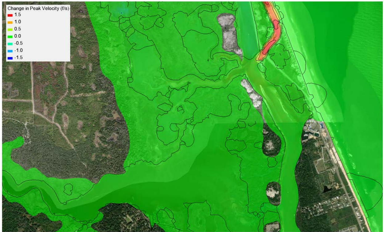
Figure 1.43 Change in Velocity within Inlet at Peak Flood Flow – Scenario 2 vs. Existing Conditions
